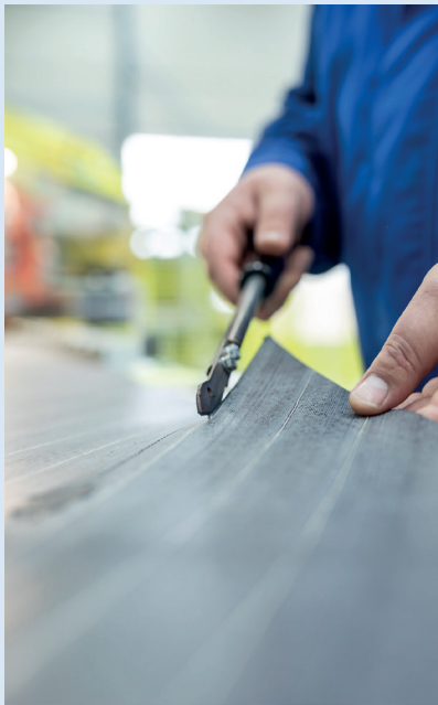
Karl Eugen Fischer manufactures machines that produce steel cord, the supporting structure of a tyre. So that the material can be cut cleanly, the cutting knife is heated.
